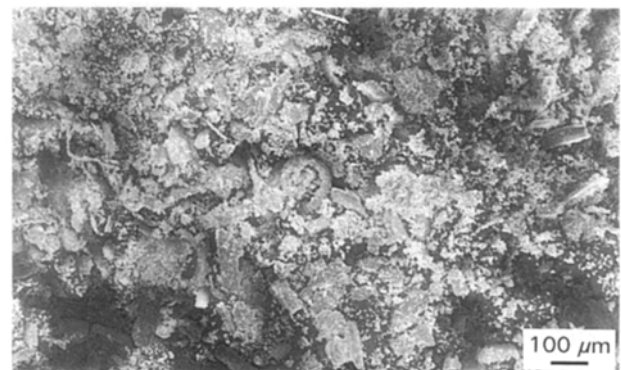
Figure 6 Scanning electron micrograph of abrasive wear debris on a 20% \text{Al}_2\text{O}_3 composite.
